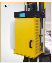
M - Mechanical brake FM - Electromagnetic brake LP - Powered prestretch 200%
